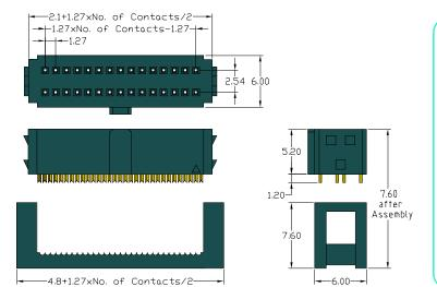
Current Rating: 1.0 Amp Withstanding Voltage: AC 500V/minute Insulation Resistance: 1000M? Min. Contact Resistance: 20M? Max. Operating Temperature:  $-40^{\circ}$  to  $+105^{\circ}$ Contact Material: Phosphor Bronze Material Insulator: PA66 (UL94V-0) Finish: Gold flash
